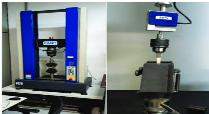
Figure 1: Universal testing machine setup (schematic). A servo-hydraulic UTM was used for tensile tests, with specimens gripped between top and bottom jaws and an extensometer attached to measure strain. This setup applies uniaxial load until failure, providing stress–strain data for each heat-treated sample.
