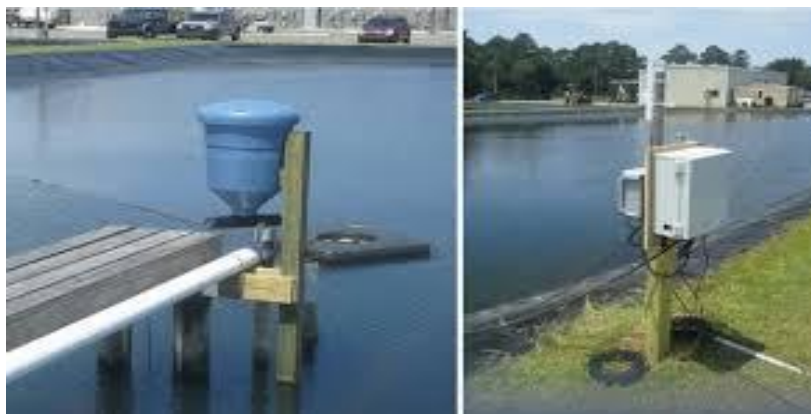
Fig.4: Automated Feeding and Monitoring Systems Source: (Global Seafood Alliance)
